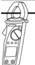
Fig. 6: Use of clamp during DC current measurement.
