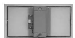
Correctly place the flat plug near the battery compartment directly into the socket.
