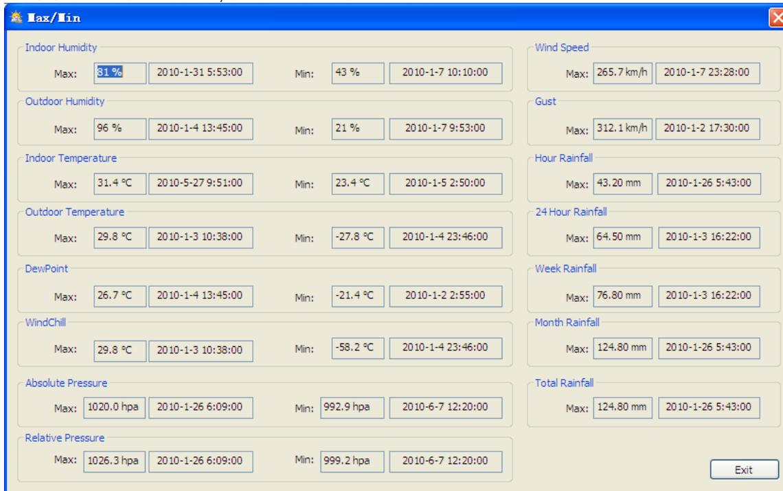
This section is used to display the recorded min and max value recorded with time stamp. Min/Max reset can only be done through key operation on the base station.
